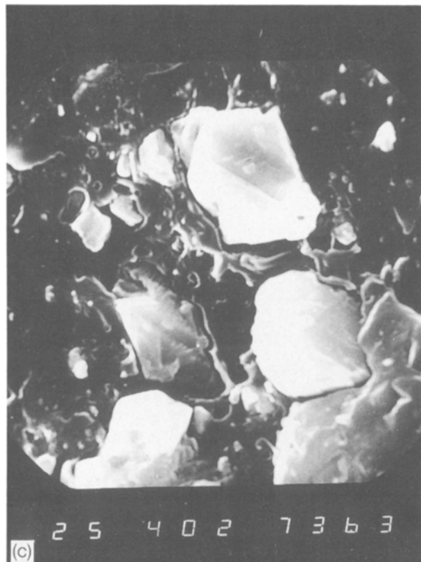
Figure 7 SEM micrographs taken from the fracture surface of PP/CaCO 3 composites deformed to different extents. Deformation: (a) 0%, (b) \epsilon_y , (c) 2\epsilon_y , (d) 5\epsilon_y (necking region). Magnifications (a) 10000, (b) 6000, (c) 4000 and (d) 3000.
